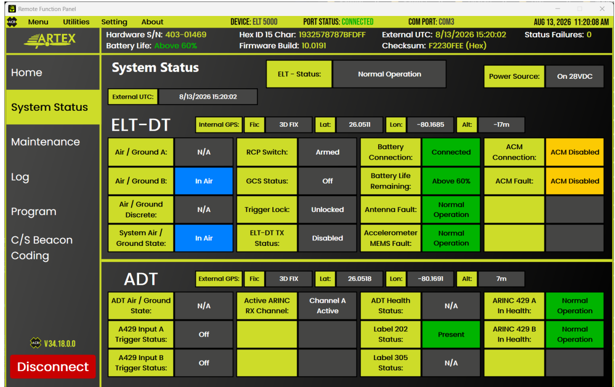
Figure 10 - RFP System Status Screen
