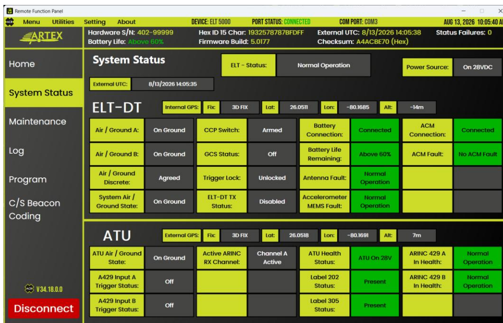
Figure 53 - RFP System Status with No Faults
