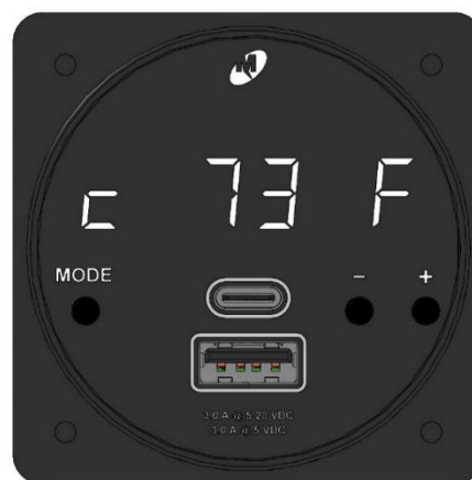
Figure 4.18 Temperature Mode Cockpit/Cabin Temperature (-5 unit shown)
