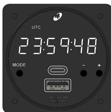
Figure 4.7 Universal Time Clock Mode (-5 unit shown)
